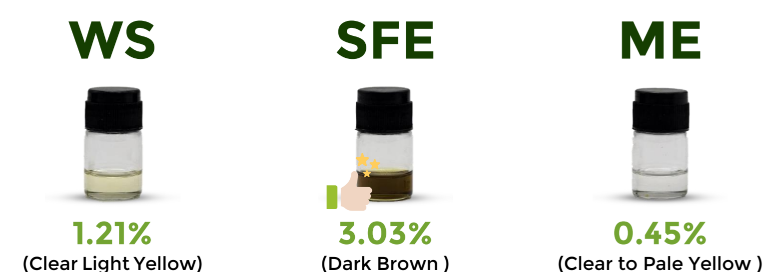
Figure 1 Yield and characteristics of lime essential oil obtained from water and steam distillation, supercritical CO 2 extraction and microwave extraction.
